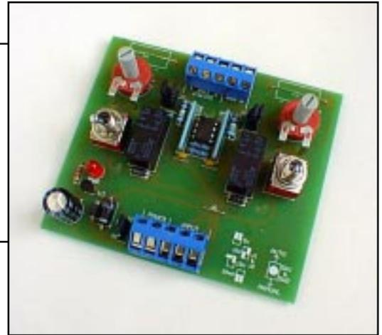
The MAO installs between a controller and an actuator to provide adjustable analog manual override when needed. In normal operation two (2) analog signals route from the controller through the MAO to each actuator. Flip the override switch from automatic to manual on either
